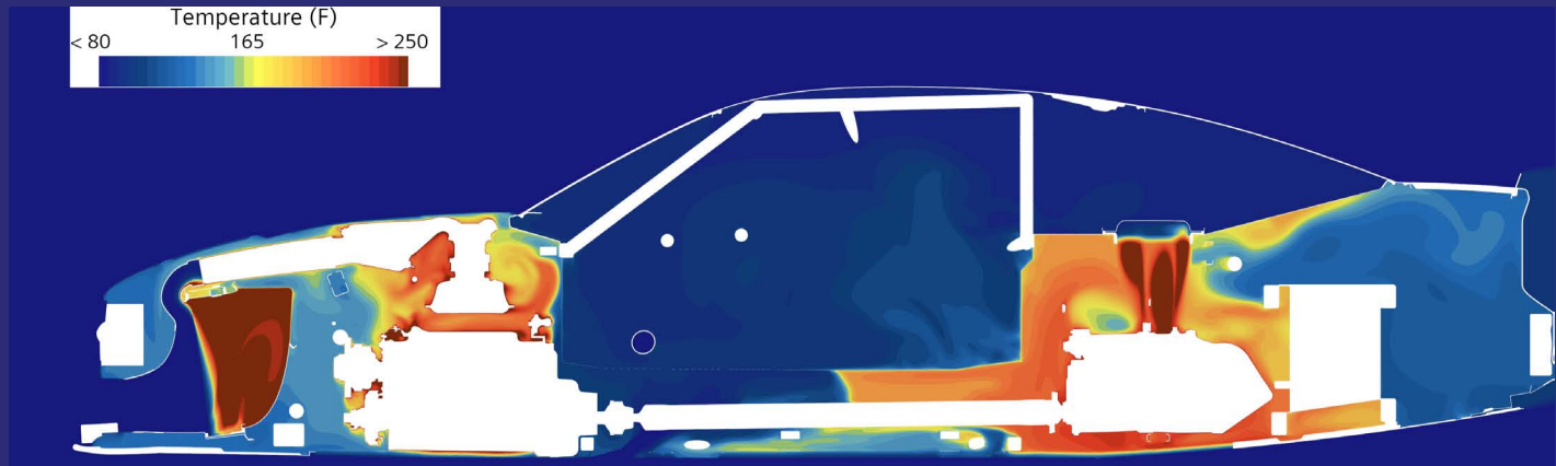
Modeling the buildup of heat in NASCAR cabins, engineers redesigned exhaust panels for better air flow, keeping drivers cool under pressure. Copyright Greg Padgett, TotalSim
