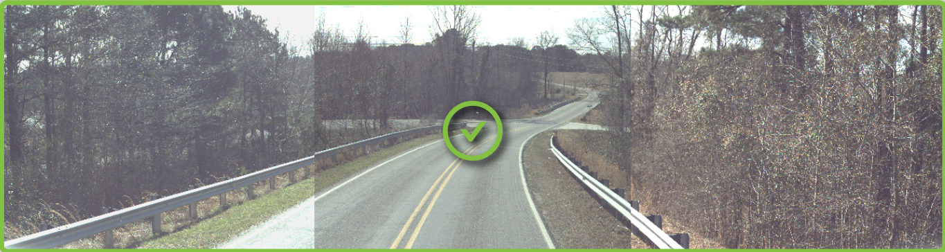
A prototype system for assessing road safety successfully detected guardrails 90% of the time (shown here) and utility poles 88% of the time. Copyright RENCi at UNC-Chapel Hill
